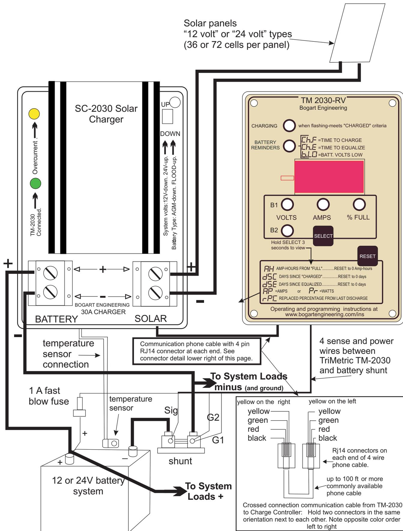
Wiring for TriMetric TM2030 and charge controller--not showing circuit breakers to battery or solar panels
